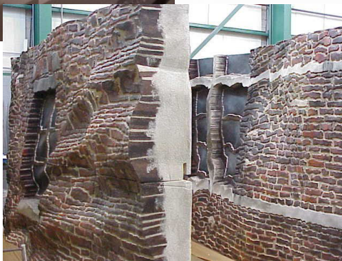
The sections are painted and sealed with an armor coat of urethane
