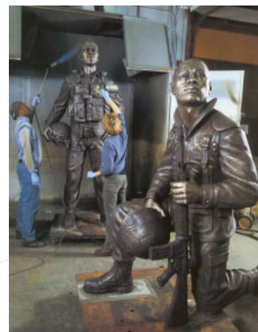
The casting of the aviator at the patina and coating station
