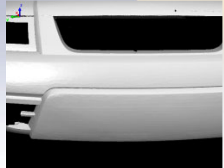
4- The Bézier surface is tessellated and the curved set of polygons is connected to the surrounding triangles.
