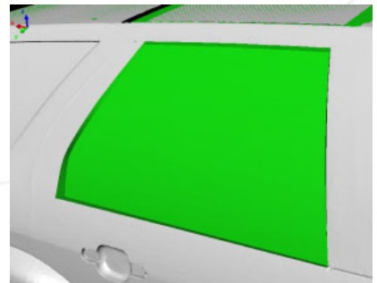
4- The tessellated surface is connected to the surrounding triangles. The model is now watertight.
